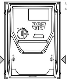
Using a suitable flat blade screwdriver, rotate the two retaining screws indicated until the screw slot is vertical.
