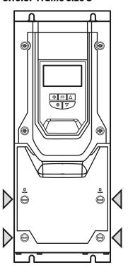
Using a suitable flat blade screwdriver, rotate the four retaining screws indicated until the screw slot is vertical.
