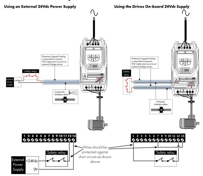
**NOTE** The Maximum cable length from Voltage source to the drive terminals should not exceed 25 mtrs.
